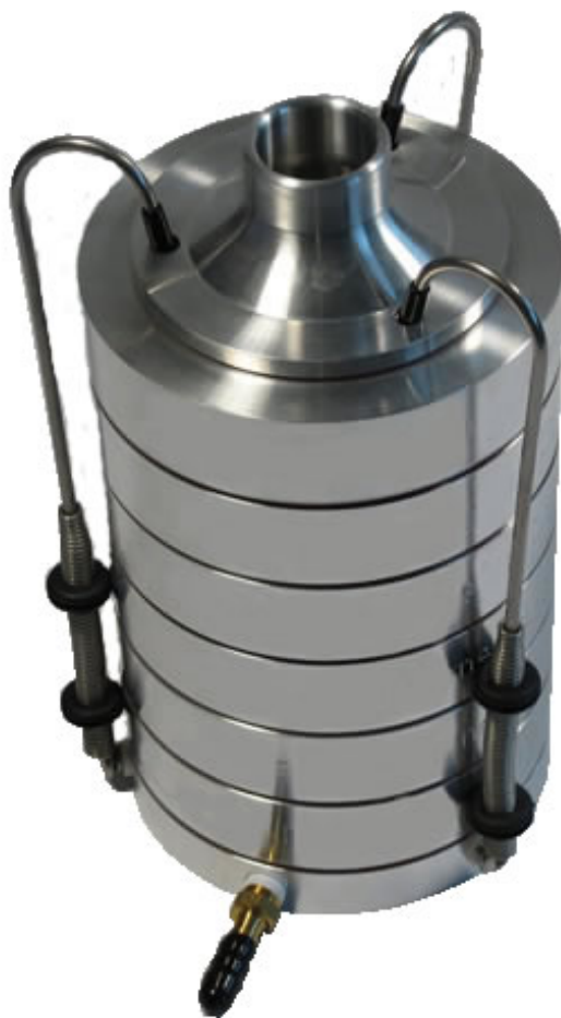
Figure 2 BGI Six-Stage Viable Sampler The jet orifice dimensions and particle size ranges for each stage are:
